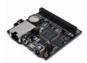
It is a wired LAN programmable board embedded with a PHPoC interpreter. It supports various interfaces to connect with sensors and equipment, and you can control your equipment from a remote site via web browser. Also, you can stack expansion boards to implement additional functions.
