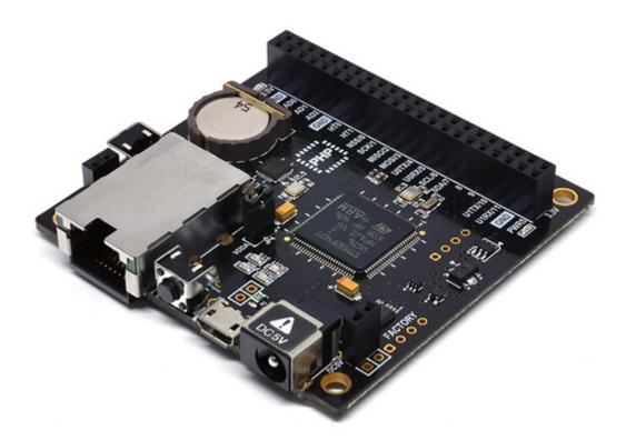
P4S-341 is an industrial programmable I/O board. You can build various network communication systems connecting P4S-341 to many devices such as sensors and actuators. We provide a self-development programming language, which is called PHPoC, for programing P4S-341. This language is easy to use and compatible with PHP which is widely used script language.
